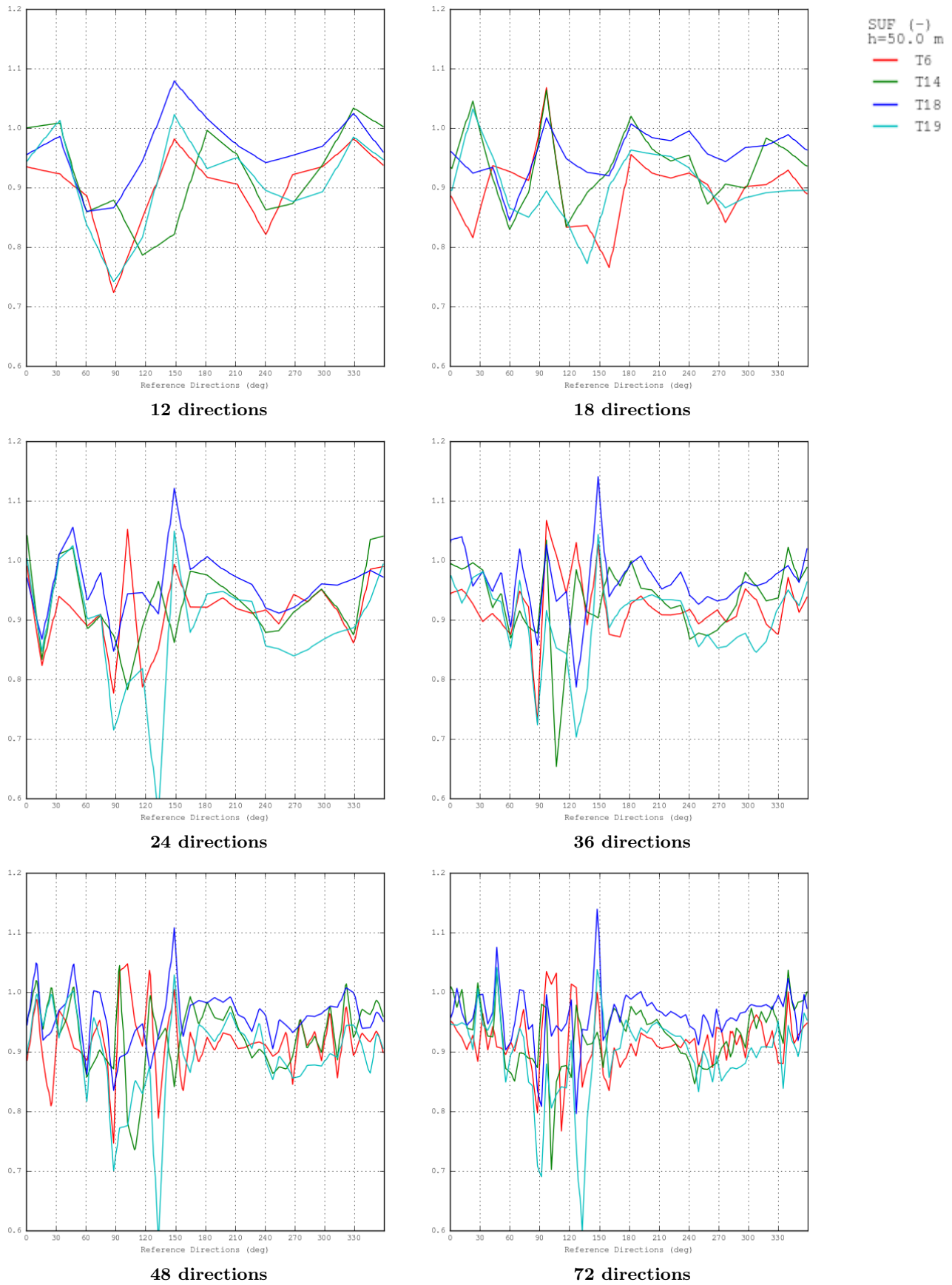
Figure 11: Speed-Up Results Interpolation against Wind Direction at Four Turbines Locations for Different Numbers of Computed Directions
