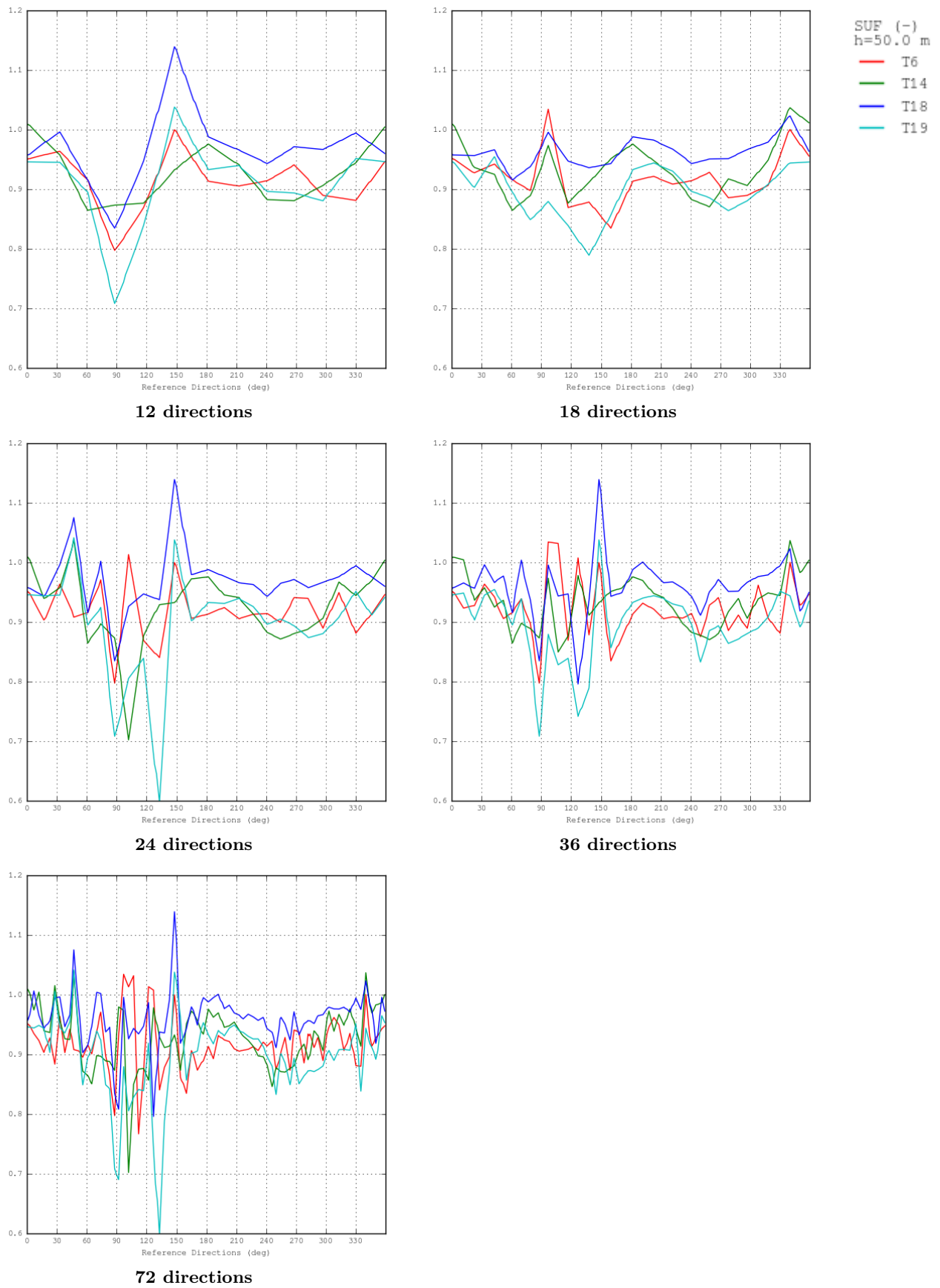
Figure 13: Speed-Up Results Interpolation against Wind Direction at Four Turbines Locations for Different Numbers of Directions Computed on the Same Mesh
